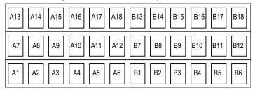
The carrier accommodates current levels up to 2 Amps per point or 8 Amps per each power and ground, and a voltage range of up to 264 VAC. Voltage transients up to 300 VAC will not damage the carrier.
